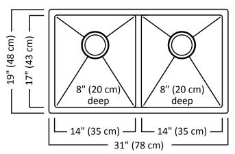
Material Construction 18 gauge, 18-10 stainless steel, type 304
