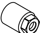
**2.** For the faucet outlet hose adapter, install a  $\frac{1}{2}$ " NPT male nipple, recessed  $\frac{3}{8}$ " behind the surface of the finished wall.
