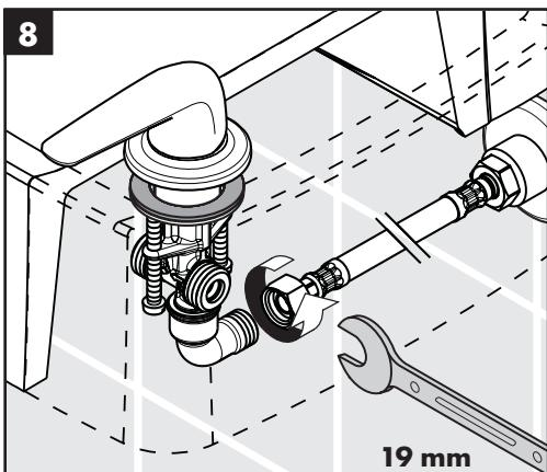
Connect the outlet hose to the elbow.
