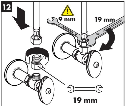
Install the adapters on the stops.
