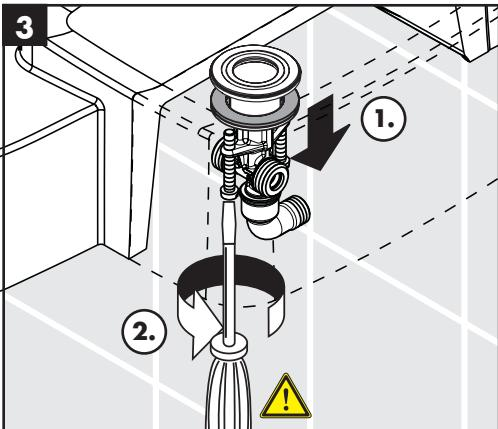
Rest the valve on the sink.
