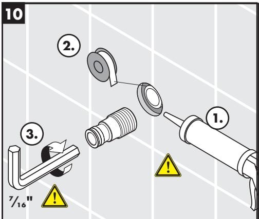
Wrap the threads on the nipple using Teflon tape.
