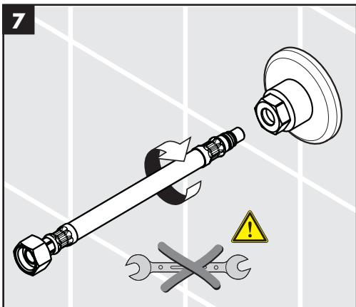
Install the outlet hose on the adapter by hand.
