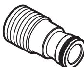
**1.** The spout uses connecting thread 96472001. The connecting thread is dual-threaded:  $\frac{3}{4}$ " male and  $\frac{1}{2}$ " female. For this installation, use the  $\frac{1}{2}$ " threads.
