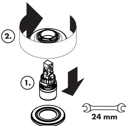
Push the cartridge into the valve.
