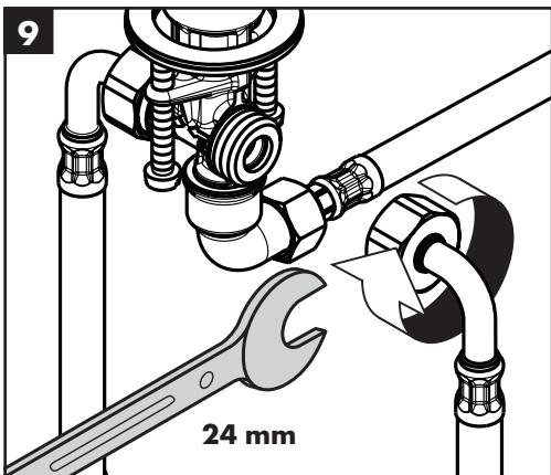
Connect the hot and cold supply hoses to the valve.
