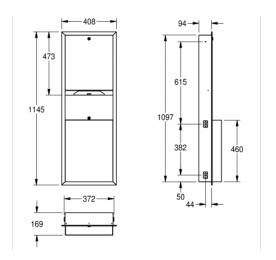
Paper towel dispenser - waste bin combination for recessed mounting, stainless steel, surface satin finished, material thickness 22 gauge folded front cover, cylinder lock with Franke standard key, loading capacity 500 - 800 pcs. of paper depending on convolution, waste bin with approx 23 litre capacity, including stainless steel screws and dowels.
