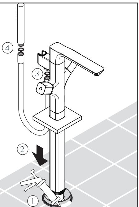
**⚠ SEAL THE FLOOR AROUND THE ROUGH USING WATERPROOF SEALANT.**
