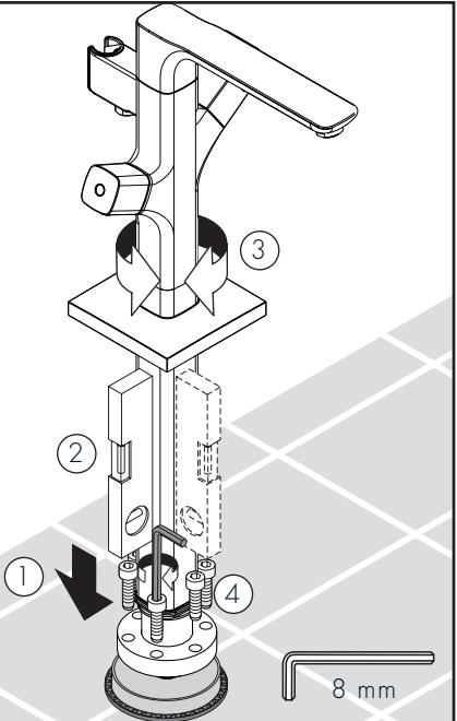
Position the tub filler on the rough. Pivot the tub filler, if necessary.
