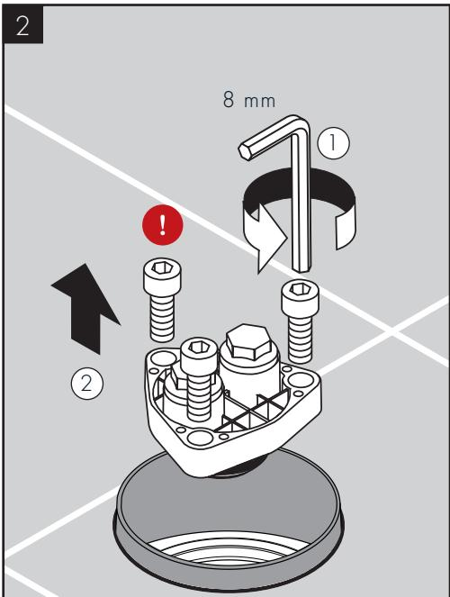
Remove the flush insert.
