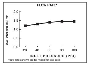
1.5 gpm/5.7 L/min. FLOW RATE
