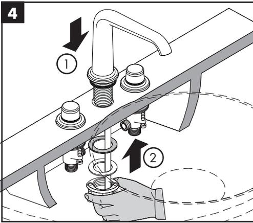
Install the fiber washer, metal washer, and mounting nut on the spout assembly.
