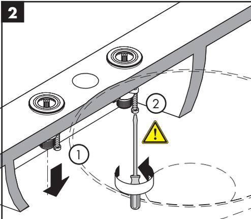
Rest the valve assembly on the mounting surface.
