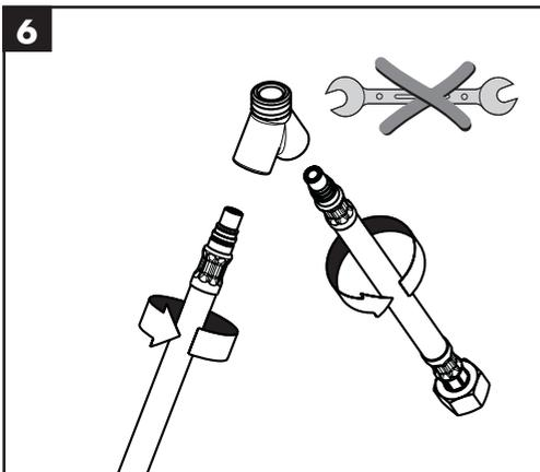
Connect the hot and cold hoses to the mounting angle by hand.
