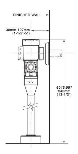
\*Note: The Critical Line (-C-L-) on Vacuum Breaker must typically be a minimum of 6" (152mm) above fixture. Consult Codes for details.
