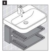
Slide the vanity under the washbasin. Tighten mounting nuts with a wrench until the washbasin is stable.
