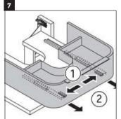
Push and lock in pins, (1) and remove the drawer. (2)
