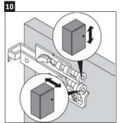
Check the vanity is leveled, and securely attached to the wall.
