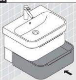
Check the vanity is leveled and make adjustments using screws.
