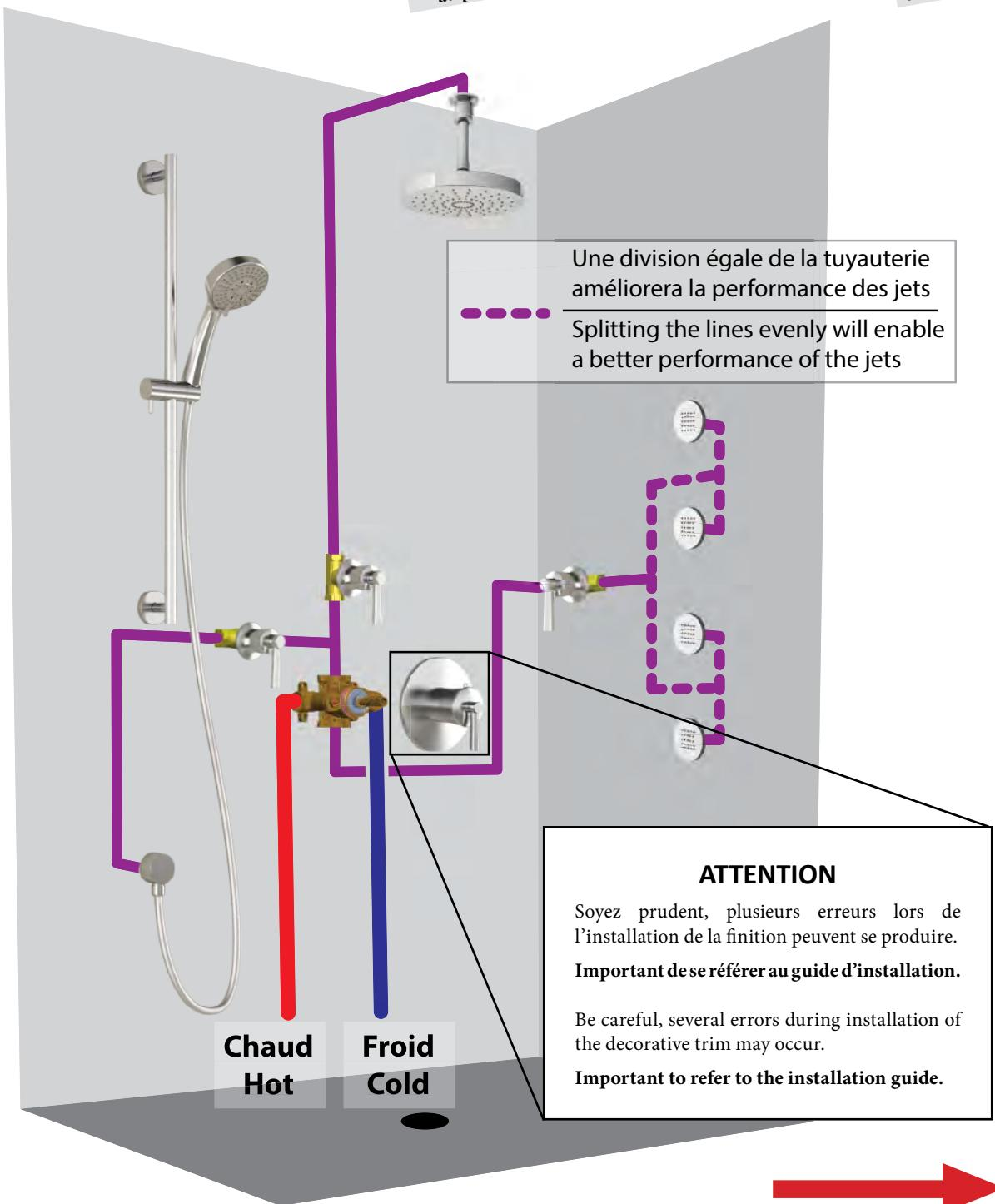
POUR UNE INSTALLATION À 2 VALVES, VOIR AU VERSO DE LA FEUILLE / FOR 2 VALVES INSTALLATION SEE BACK OF SHEET
