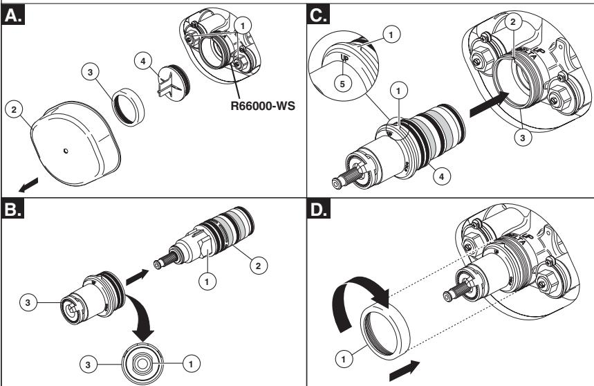
**Note:** The Sensori® Thermostatic Valve rough (R66000-WS) must be installed before installing the trim.
