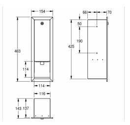
Soap dispenser for recessed mounting, stainless steel, surface satin finished, material thickness 20 gauge folded front cover, cylinder lock with Franke standard key.
