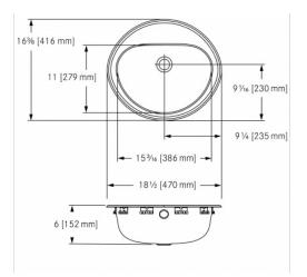
Single compartment self rimming vanity basin with faucet ledge. 18 gauge (1.2 mm), type 304 (CNS 18/10) stainless steel. Mirror finished rim, #4 satin finished bowl. Undercoated to reduce condensation and resonance. Includes factory applied rim seal, cutout template, and installation hardware. Certified to ASME A112.19.3-2008 / CSA B45.4-08.
