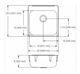
Single compartment self rimming drop-in sink with faucet ledge. 20 gauge (0.9 mm), type 302 (CNS 18/8) stainless steel. Exposed surfaces are #4 satin finished. Undercoated to reduce condensation and resonance. Includes factory applied rim seal, cutout template, and factory installed EZ TORQUE™ fasteners. Certified to ASME A112.19.3-2008 / CSA B45.4-08
