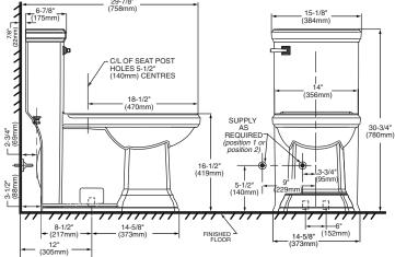
IMPORTANT: Water supply on the wall is required at 3-3/4" (95mm) or 9" (229mm) from centreline of the toilet (see rough-in). First suggested position is hidden behind the toilet. The geometry of the toilet gives space for this installation. The second suggested position is next to the toilet. Between these two positions, the space for the supply between wall and toilet is limited to 3-1/4" (83mm). In this case, check your supply and hose dimensions.
