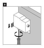
Using a screwdriver adjust the vanity mounting hinge system counter-clockwise.
