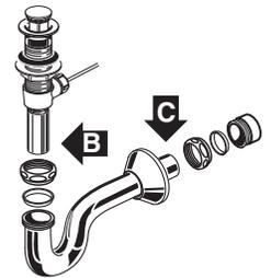
Connect hot and cold supply lines to the shut off valves. Tighten trap joints for watertight assembly.
