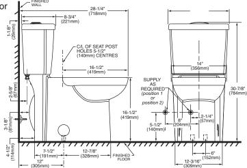
IMPORTANT: Water supply on the wall is required at 2-1/4" or 8" (57 or 203mm) from centreline of the toilet (see rough-in). First suggested position is hidden behind the toilet. The geometry of the toilet gives space for this installation. The second suggested position is next to the toilet. Between these two positions, the space for the supply between wall and toilet is limited to 4-1/2" (114mm). In this case, check your supply and hose dimensions.
