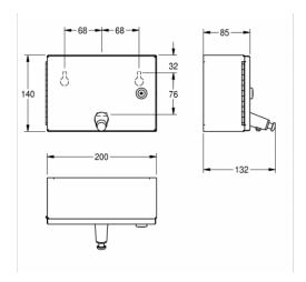
Soap dispenser for wall mounting, stainless steel, surface satin finished, material thickness 20 gauge folded front cover, cylinder lock with Franke standard key.
