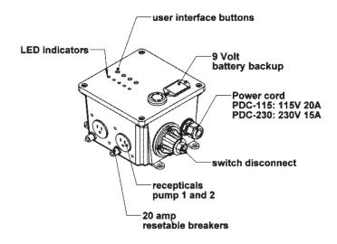
PDC-series controllers feature a programmed 6 hour run limiter for pump protection. If the alarm float remains closed (up position) for 6 hours but the primary float switch is open (down position) the alarm light will flash and the pump is turned off. This feature prevents the pump from running indefinitely and protects against run-dry situations.
