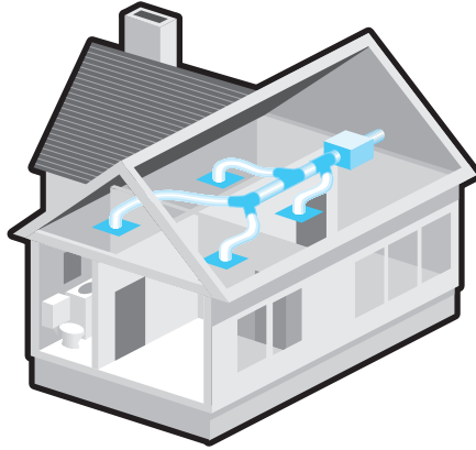
Continuous (low rate) ventilation with multiple inlets through the home for indoor air quality improvement
