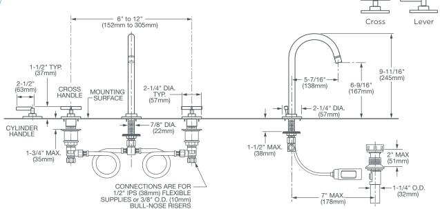
NOTE: MOUNTING HOLES ARE 1-3/8" DIA. (35mm)
