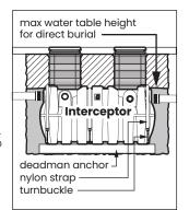
Model GB-500 uses model AK2 anchor kit for use with deadmen anchors.
