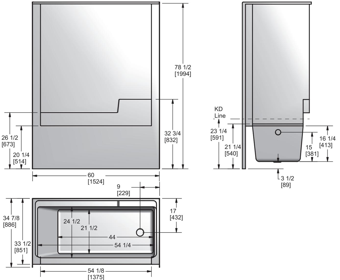
Measurement tolerances ± 1/4" (6.3 mm)
