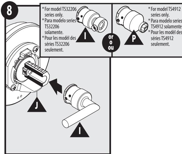
Install Lever Handle (I) onto Adapter (J) as shown.
