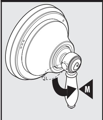
Rotate Handle Insert (M) 90° counter-clockwise so that handle insert faces down.
