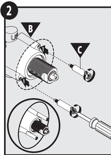
1. Install Standoff Screws (C) into Valve (B) tabs as shown.
