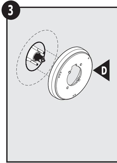
Install Escutcheon (D) onto valve stem and wall.
