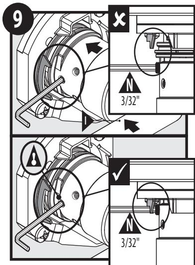
1. To tighten Lever Handle (I) engage the 3/32" Hex Wrench (N) to set screw and push lever handle inward towards bracket.
