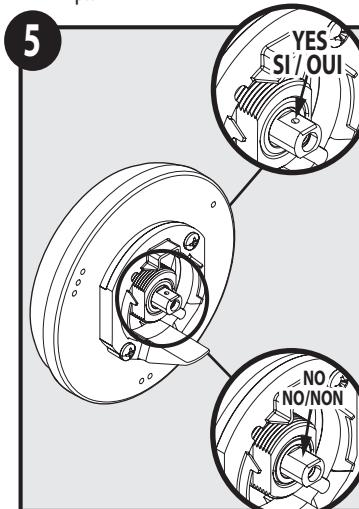
Ensure cartridge stem with notch indentation is facing towards the 9 o'clock position. See inset for correct orientation.
