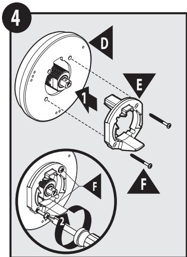
1. Attach Mounting Bracket (E) to Escutcheon (D).
