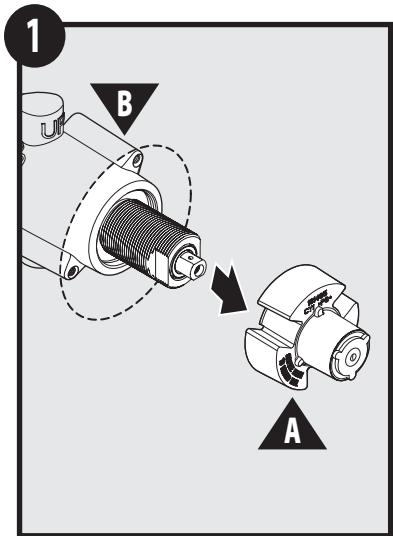
Remove Plaster Ground (A) from Valve (B) through wall opening to begin trim installation.
