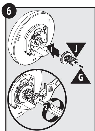
1. Install Adapter (J) and Adapter Screw (G) onto bracket.
