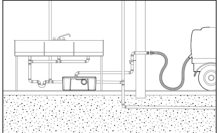
**At Grade Under Sink Installation with Outdoor Remote Pumpout Hook-up**
