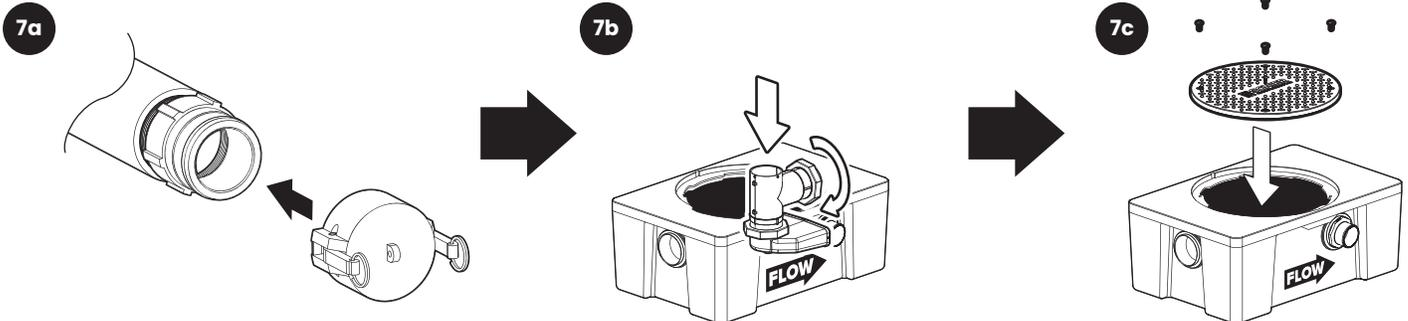
Install Cam and Groove Cap at hookup
