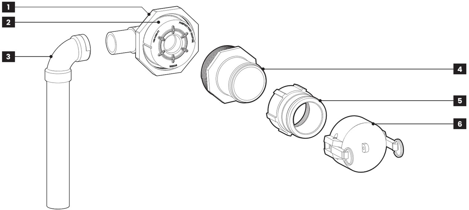
1. Pumpout Adapter Retaining Nut
