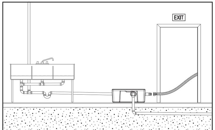
**At Grade Same Floor Installation with On-site Pumpout Hook-up**
