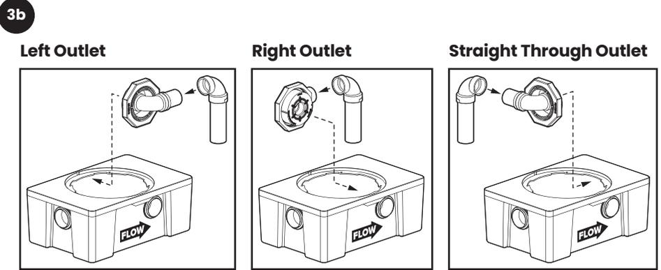
Dry fit pumpout adapter and vertical pipe assembly as shown for chosen port location (Left, Right or Straight Through). Hand tighten into place. Ensure that vertical piping assembly is pointed down (as shown) and ensure that there is at least 1/2" of clearance between the vertical pipe and floor of unit. Remove internal piping assembly for cementing.
