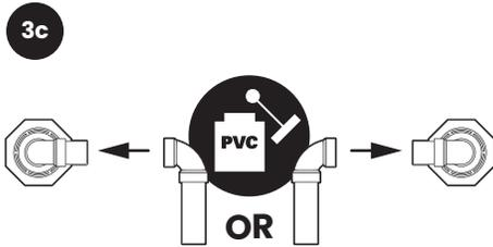
Use PVC primer/cement to secure pumpout adapter to vertical pipe assembly.
