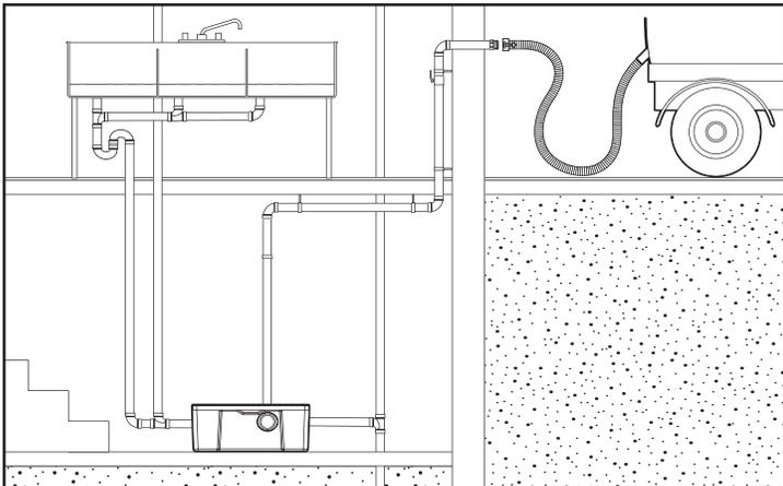
**At Grade Basement Installation with Outdoor Remote Pumpout Hook-up**
