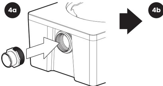
Install the supplied 3" plain end fitting at the pumpout port using pipe thread sealant or tape.
