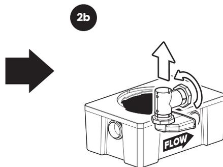
Unscrew diffuser retaining nut and remove outlet diffuser.
