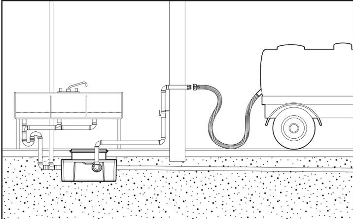
**Below Grade Installation with Outdoor Remote Pumpout Hook-up**
