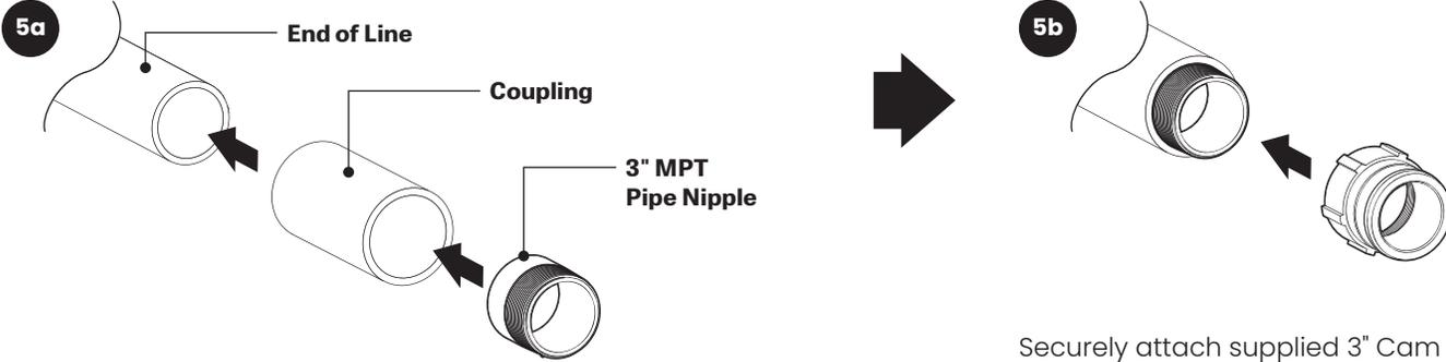
At the end of the pumpout plumbing line, install a 3" MPT pipe nipple (Not included with this kit) using a coupling of your choice.
