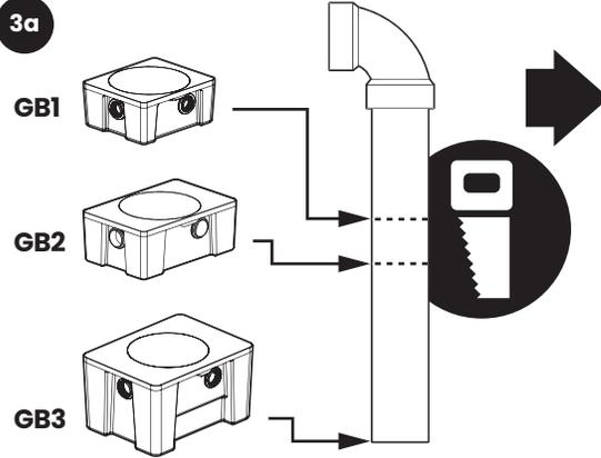
Trim internal vertical piping assembly at premarked location.
