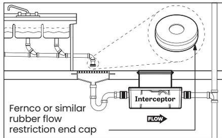
See drawing for guidance. For detailed guidance on indirect connections, go to: [webtools.schierproducts.com/Technical\\_Data/Indirect\\_Connections.pdf](http://webtools.schierproducts.com/Technical_Data/Indirect_Connections.pdf)
