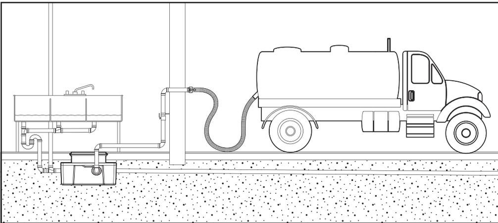
Run Sinks to ensure interceptor is full of water. Attach pumper hose to 3" cam and groove fitting. Turn on pump, make sure interceptor is pumped out and inspect pumpout plumbing for leaks.
