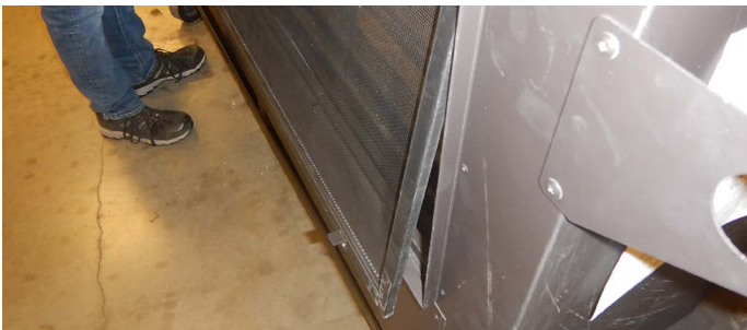
Figure 20.b Lift out the Retaining Tabs and screen
