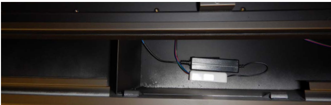
Figure 25.a. Secure LED receiver
