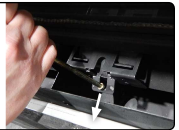
Figure 21.d Pull door latches
