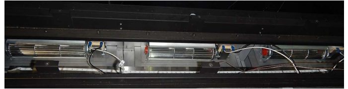
Figure 27.d secure the fans
