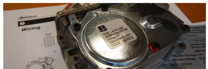
Figure 13.k Conversion label on valve
