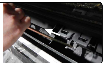
Figure 21.d Pull door latches
