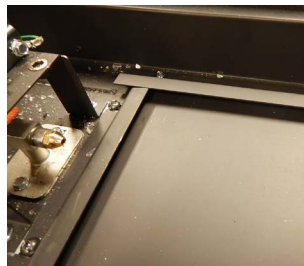
Figure 12.f Unscrewing brackets securing metal plate
