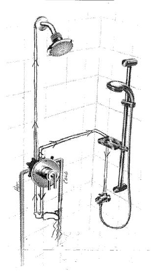
To add a tub spout to the dual function Grohflex (either PBV or Thermostatic), plumb the hand shower connection from the top of the Grohflex valve. The from the bottom, plumb down into the  $\frac{1}{2}$  inlet on a Twin Ell (03671000). From the  $\frac{3}{4}$  outlet on the twin Ell go into a Diverter tub spout. From the  $\frac{1}{2}$  outlet on the Twin Ell go up to the shower head.
