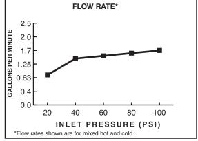
1.83gpm/8.3L/min. FLOW RATE
