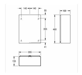
Waste bin for wall mounting, stainless steel, surface satin finished, material thickness 22 gauge rounded edges, mounting either with mounting bracket or directly onto the wall, including stainless steel screws and dowels.
