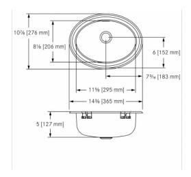
Single compartment self rimming vanity basin less faucet ledge. 18 gauge (1.2 mm), type 304 (CNS 18/10) stainless steel. Mirror finished rim, #4 satin finished bowl. Undercoated to reduce condensation and resonance. Includes factory applied rim seal, cutout template, and installation hardware. Certified to ASME A112.19.3-2008 / CSA B45.4-08.
