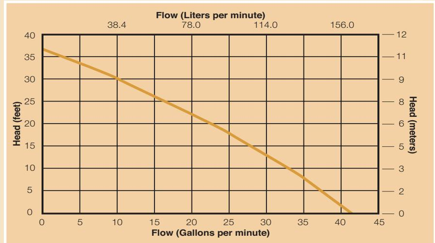
**Note:** Maximum shut-off head is 36 feet. Usable maximum head - assuming 150' of lateral discharge through 1" pipe is 25 feet. Consult factory for proper sizing and calculation of friction loss.
