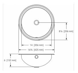
Single compartment self rimming vanity basin less faucet ledge. 18 gauge (1.2 mm), type 304 (CNS 18/10) stainless steel. Mrror finished rim, #4 satin finished bowl. Undercoated to reduce condensation and resonance. Includes factory applied rim seal, cutout template, and installation hardware. Certified to ASME A112.19.3-2008 / CSA B45.4-08.
