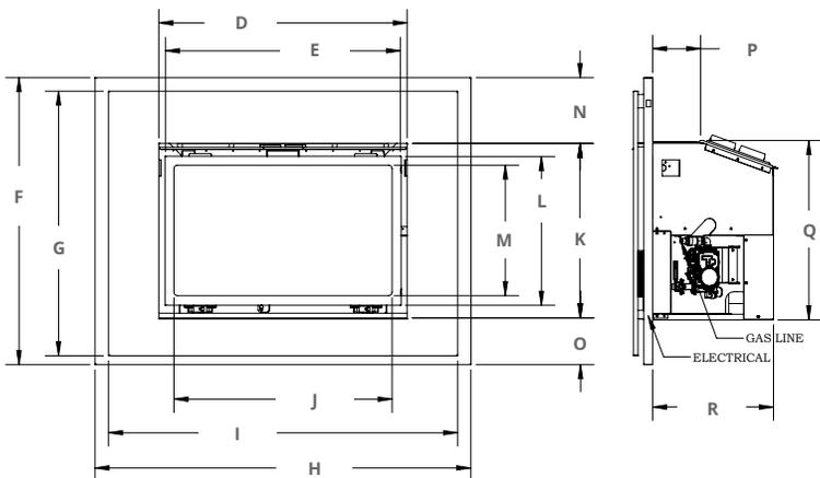
Figure 1.6 Unit dimensions (Tolerance  $\pm \frac{1}{8}$ ") [1.25 mm]
