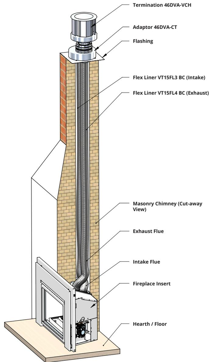
Figure 3.1 Vent Configurations
