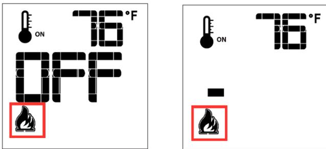
Figure 9.14 Flame Off and Flame Level 1.
