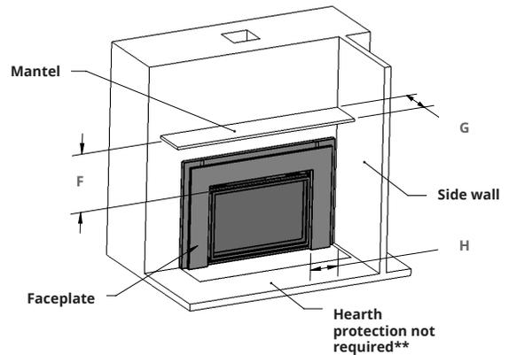
Figure 2.1 Install clearances
