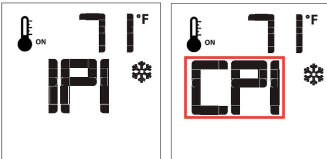
Figure 9.12a Continuous Pilot / Intermittent Pilot Selection
