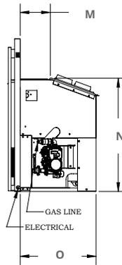
Figure 1.3 Unit dimensions (Tolerance  $\pm \frac{1}{8}$ ") [1.25 mm]
