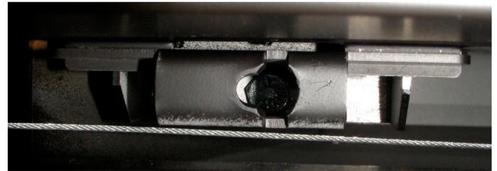
Engage door tool into door retainer. Pull door tool towards you and push downwards, disengaging the door retainer from the door.
