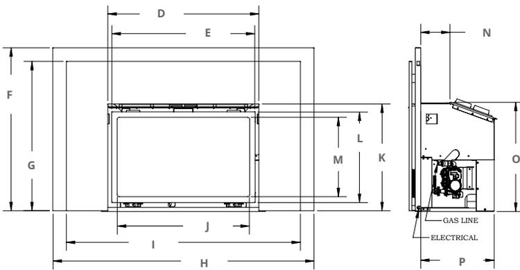
Figure 1.5 Unit dimensions (Tolerance  $\pm \frac{1}{8}$ ") [1.25 mm]
