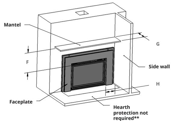
Figure 2.1 Install clearances
