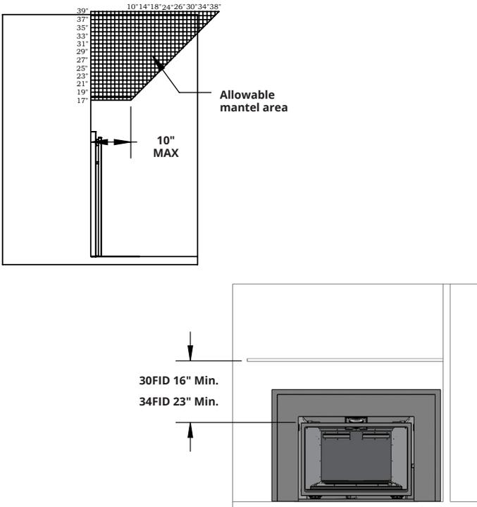
Figure 2.2 Install clearances
