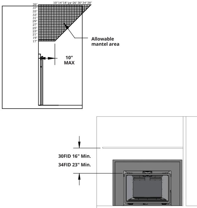
Figure 2.2 Install clearances
