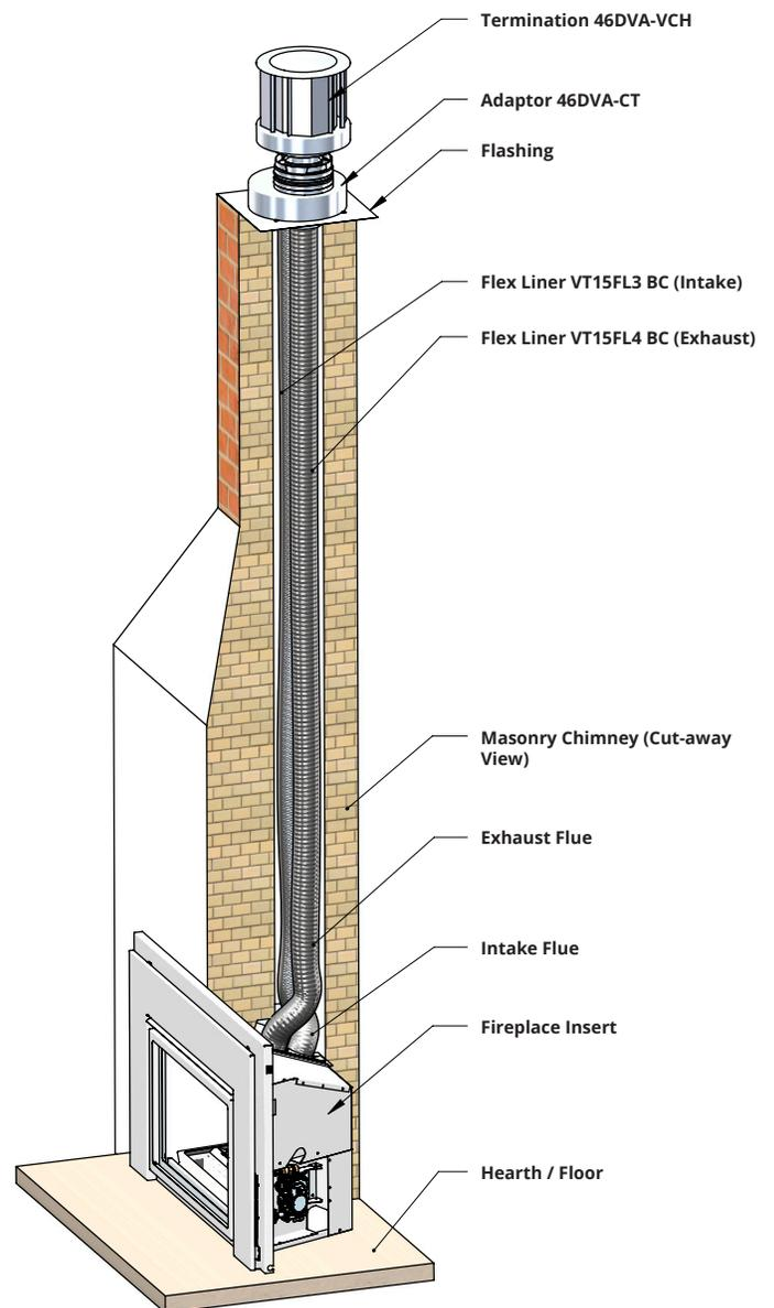
Figure 3.1 Vent Configurations
