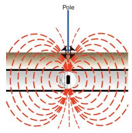
The RIDGID NaviTrack FloatSonde floats with the Pole pointing straight up. Some other floating Sondes float with the Sonde axis in line with the pipe. To locate a Sonde in a vertical orientation, center the Pole icon in the Active View Area. For vertical Sondes, only one pole is found above ground.
