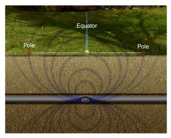
6. To verify you have located the Sonde, make sure the Signal Strength drops when you move the receiver in any direction.
