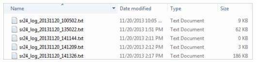
5. Open the desired data log file. The data log file should automatically open in Notepad or your default text editor. In the data log file, the first line is the header and the lines that follow contain the logged data.
