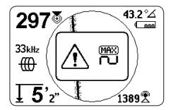
The SR-24 responds to clipping by attenuating the measurement. Attenuation reduces the intensity of the Signal Strength so the SR-24 can measure it. If the SR-24 is still experiencing clipping, increase the distance between the SR-24 and the target line.
