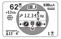
Note: You can tune the SR-24 to a frequency by watching the Signal Strength in the lower right of the screen while adjusting the frequency.
