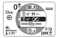
The signal that is closest to the receiver is the primary signal and its frequency range is displayed above the OmniSeek icon on the screen. The bold Tracing Line and other display readings will reflect its characteristics.
