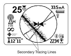
Secondary Tracing Lines make it easier to detect the presence of multiple utilities. If one or two Secondary Tracing Lines appear out of alignment with the Tracing Line, there may be another utility in the area. Secondary Tracing Lines that are out of alignment could also indicate the presence of signal energy on the same utility in different frequency bandwidths.
