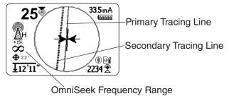
If the SR-24 detects signals in the other two frequency ranges, it displays dashed Tracing Lines to indicate the estimated position of these secondary signals. If the receiver is moved, focus automatically shifts to the closest signal.
