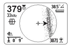
You can set the Tracing Line Distortion Response to high "H," medium "M," low "L" (default), or "OFF." Set the Tracing Line Distortion Response to high to increase its sensitivity to distortion.
