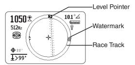
The Race Track is the circular track around the Active View Area. As you move the receiver, the Level Pointer moves clockwise around the Race Track as Signal Strength increases and regresses counterclockwise when the Signal Strength decreases. When the Signal Strength begins to decrease, a Watermark is left behind to represent the highest signal level detected.
