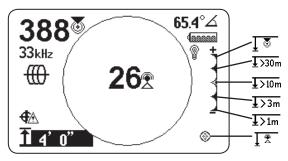
Note: The depth measurement appears on a black background when the SR-24 is measuring a negative depth (signal from above the SR-24).
