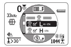
With a broadband signal type, the SR-24 displays positional information for the strongest source in the given frequency range.
