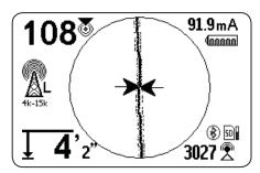
The Guidance Line gets longer as the receiver aligns with the direction of the target line. For best guidance accuracy, align the Tracing Line and Guidance Line between the Guidance Arrows. As a general rule, if there is a moderate mismatch between the Tracing Line and Guidance Line, the Guidance Line will be closer to the actual utility position. Any mismatch is an indication of distortion.
