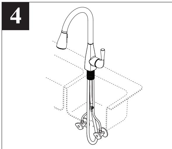
**1 Shut off water supplies.** Remove old faucet. Set new faucet into place. Push faucet as far back on sink as possible. Secure with washer (1) and threaded bracket (2). Hand tighten bracket (2) onto shank (3). Lock bracket into position by tightening screws (4).
