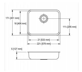
Single compartment undermount sink. 18 gauge (1.2 mm), type 304 (CNS 18/10) stainless steel. Exposed surfaces are #4 satin finished. Undercoated to reduce condensation and resonance. Includes waste fitting, cutout template, and installation hardware. Certified to ASME A112.19.3-2008 / CSA B45.4-08. Wheelchair accessible: meets ADA (Americans with disabilities act guidelines) and ANSI A117.1 (Accessible and usable buildings and facilities). Check local codes to ensure compliance.
