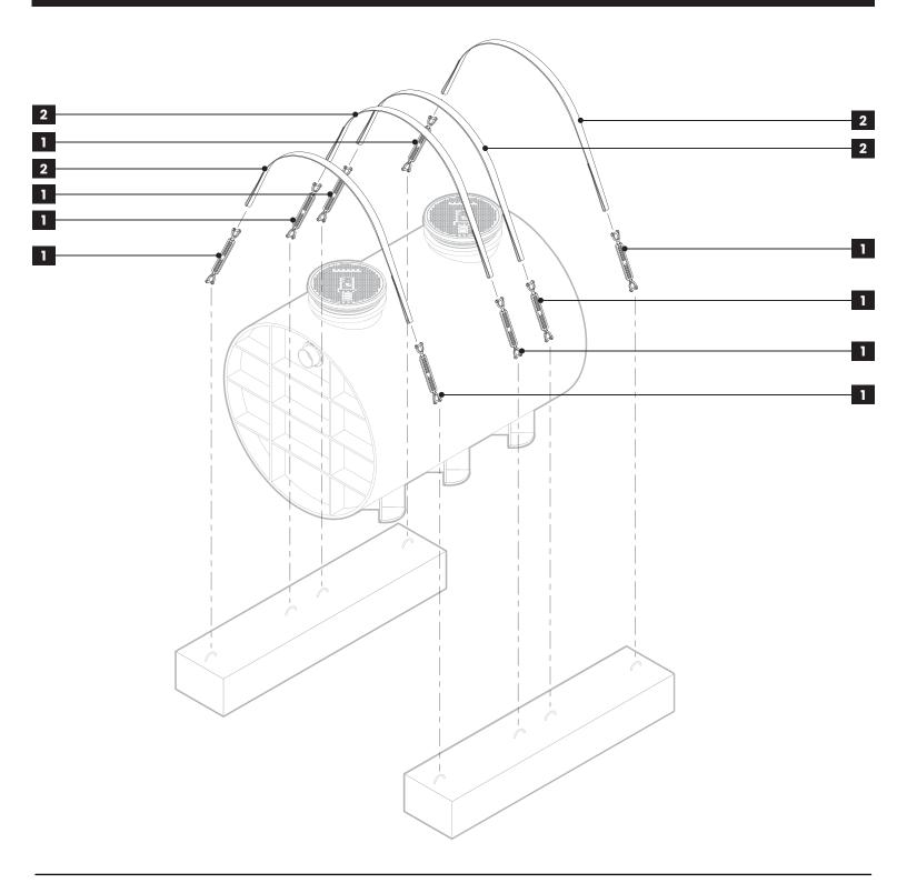
1. Jaw-Jaw Galvanized Turnbuckle (x8) 2. Polyester "Over-Tank" Straps (x4)
