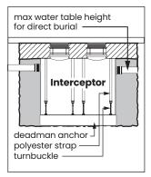
high water table scenarios must be installed with an anti-flotation anchor kit. Models GB-50, GB-75, and GB-250 use model AK1 anchor kit. Model GB-500 uses model AK2 anchor kit for use with deadmen anchors. Models GB-1000, GGI-750 and GGI-1500 use model AK3 anchor kit for use with deadmen anchors.
