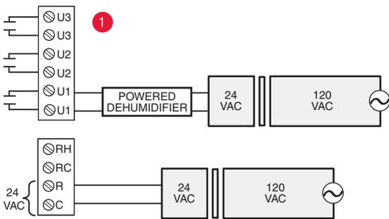
**Fig. 346. Wiring a powered dehumidifier (whole house dehumidifier).**
