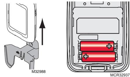
Replace batteries in your outdoor sensor when a warning appears on the thermostat screen, about two months before batteries are depleted. After new batteries are installed, the outdoor sensor will restore communication with the wireless network within a few seconds.
