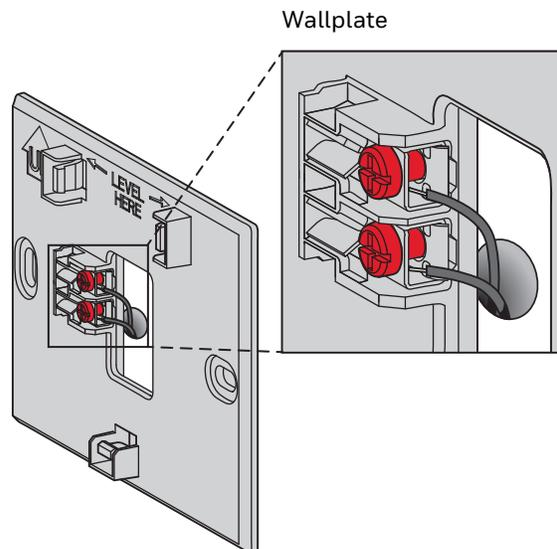
**Fig. 322. Inserting wires in thermostat terminal block.**
