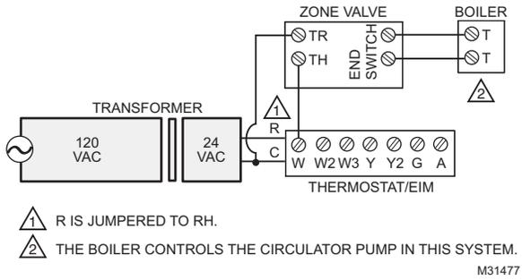
**Fig. 333. 2-Wire Zone Valve with end switch.**
