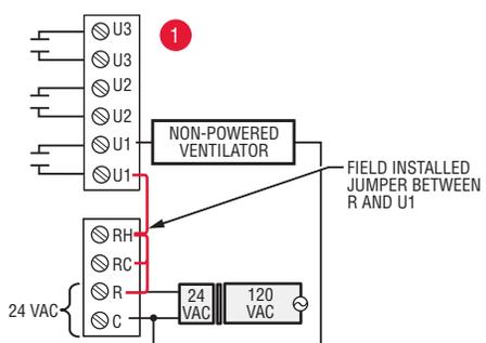
**Fig. 348. Wiring a non-powered ventilator.**
