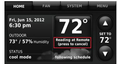
**Fig. 313. Reading temperature at the Portable Comfort Control.**
