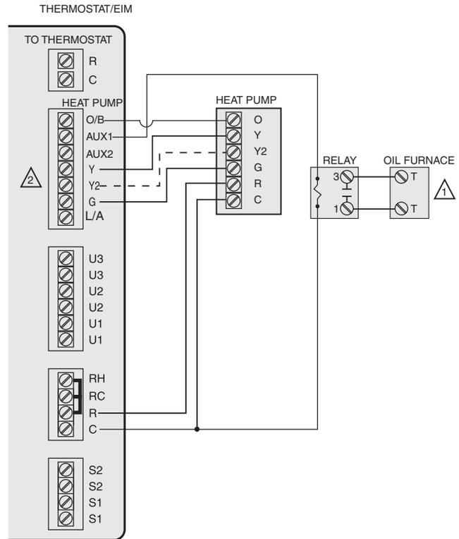
**Fig. 336. Heat pump with oil forced air backup.**
