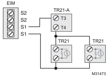
Fig. 358. Wiring 2 TR21 sensors and 1 TR21-A sensor.
