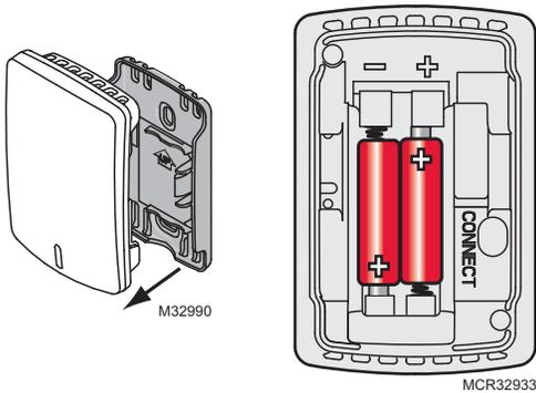
Replace batteries in your indoor sensor when a warning appears on the thermostat screen, about two months before batteries are depleted. When the sensor status light begins flashing red, battery power is critically low and will be depleted within 2–3 weeks. During normal operation, the status light remains off. After new batteries are installed, the indoor sensor will restore communication with the wireless network within a few seconds.
