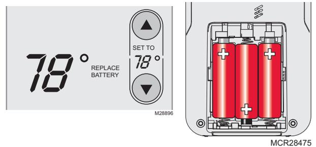
Install fresh batteries when the REPLACE BATTERY warning flashes on the screen. This warning will flash for approximately two months before the batteries fail.
