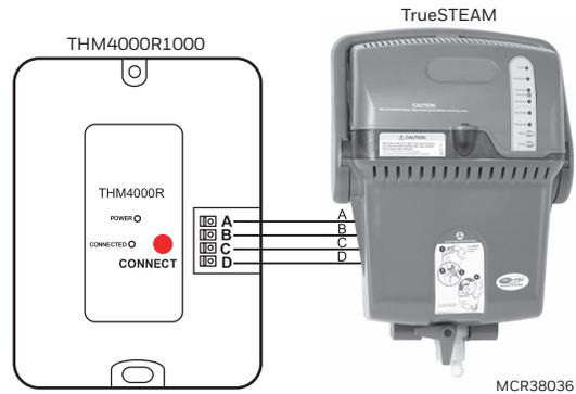
**Fig. 48. Connect button on TrueSTEAM wireless adapter.**
