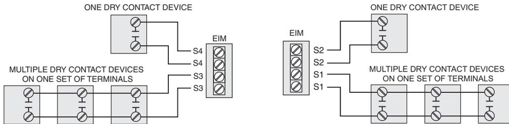
Fig. 187. Wiring dry contact devices.
