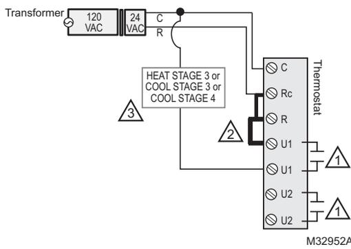
**Fig. 331. Prestige THX9321 powering relay with system transformer.**
