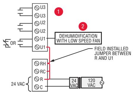
**Fig. 349. Wiring a low speed fan for dehumidification.**
