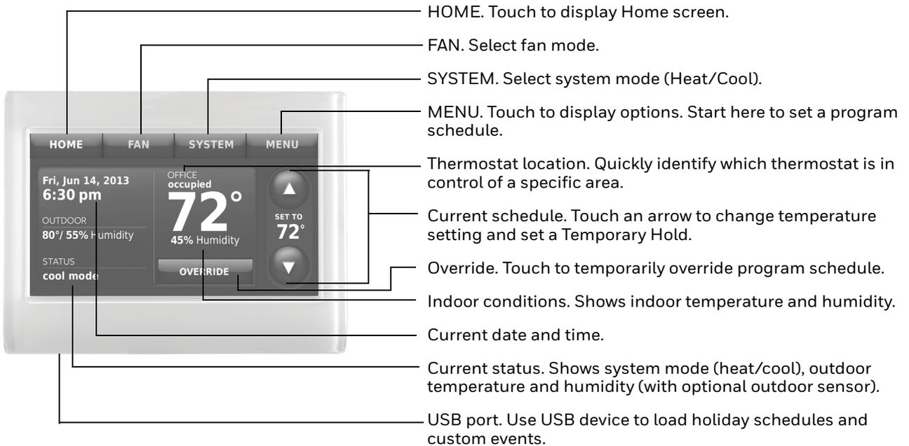
**Fig. 75. Quick reference to commercial display.**
