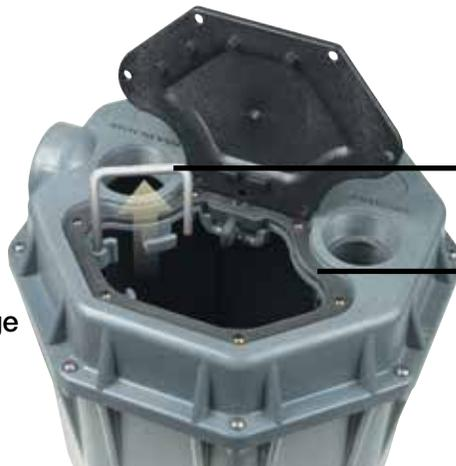
QuickTree® technology allows easy removal of float without disconnecting plumbing or pulling the pump.
