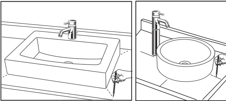
Before applying the sealant, place the sink temporarily into the cut-out. Check for alignment and clearance. Then mark the sink *and* countertop in several places as a guide for the installation location.
