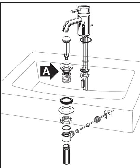
Mount the faucet and drain assembly (not included) on the sink or on the countertop following the manufacturer's instructions. Be certain to apply a bead of sealing putty on the underside of the drain (Part "A") in order to ensure a watertight seal between the sink and drain. Remove excess putty after installing drain on sink.
