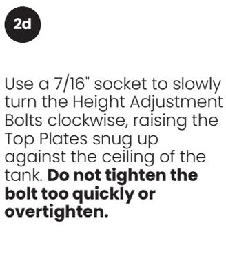
Use a 7/16" socket to slowly turn the Height Adjustment Bolts clockwise, raising the Top Plates snug up against the ceiling of the tank. **Do not tighten the bolt too quickly or overtighten.**
