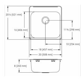
Single compartment self rimming drop-in sink with faucet ledge. 20 gauge (0.9 mm), type 302 (CNS 18/8) stainless steel. Exposed surfaces are #4 satin finished. Undercoated to reduce condensation and resonance. Includes factory applied rim seal, cutout template, and factory installed EZ TORQUE™ fasteners. Certified to ASME A112.19.3-2008 / CSA B45.4-08
