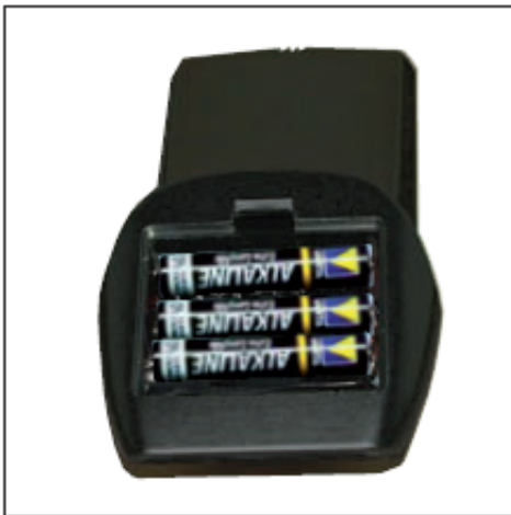
Figure 38. Remote Control Battery Compartment
