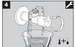
Turn the faucet on and let the water run for at least 20 seconds to ensure the lines and the faucet are flushed.
