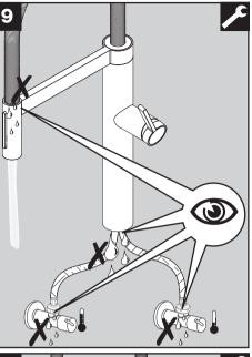
Double check all connections for leaks.
