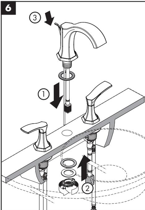
Install the drain pull rod on the spout.
