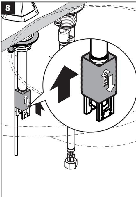
Open the quick-connect by pushing it upwards.
