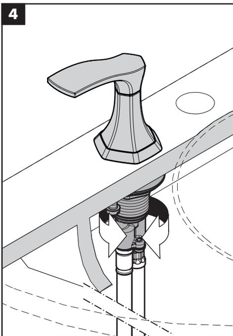
If necessary, rotate the valve.
