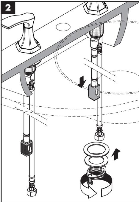
Install the fiber washer, metal washer, and mounting nut.
