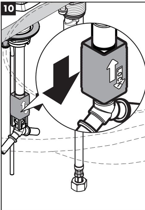
Lock the quick-connect by pulling down on it.
