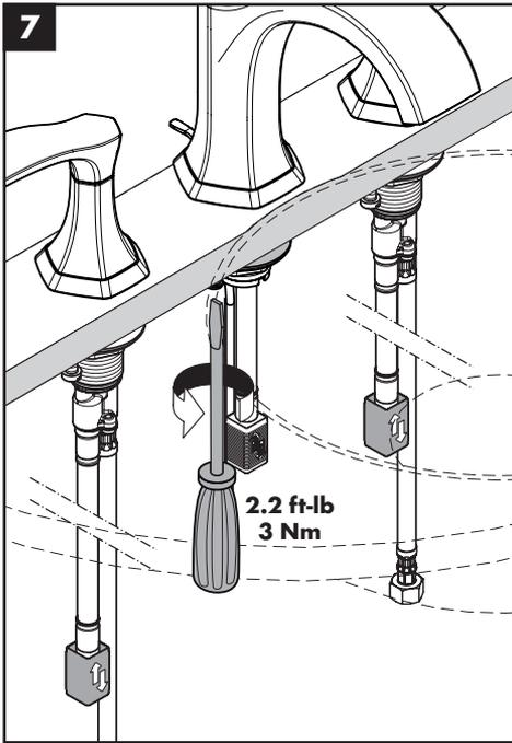
Tighten the mounting nut and the tensioning screws.
