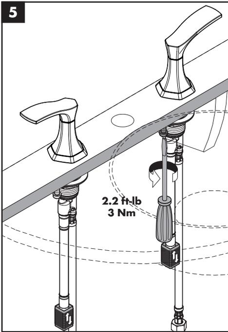
Tighten the nut. Tighten the tensioning screws.
