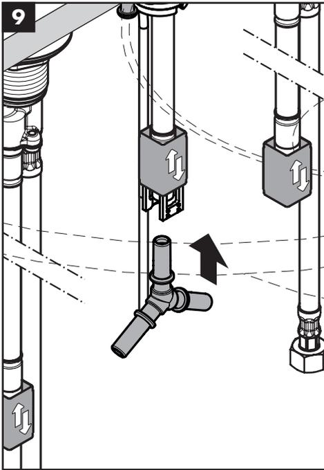
Insert the connection angle in the spout quick-connect.
