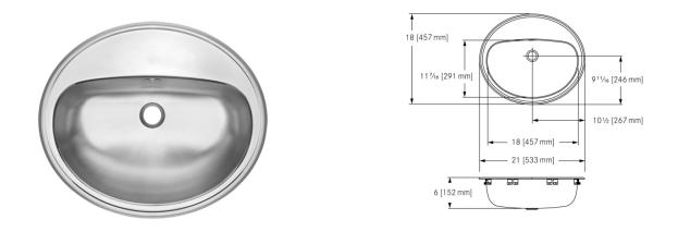
Single compartment self rimming vanity basin with faucet ledge. 18 gauge (1.2 mm), type 304 (CNS 18/10) stainless steel. Mirror finished rim, #4 satin finished bowl. Undercoated to reduce condensation and resonance. Includes factory applied rim seal, cutout template, and installation hardware. Certified to ASME A112.19.3-2008 / CSA B45.4-08.
