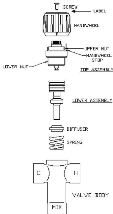
1. Pierce center circle of nameplate with a screwdriver and remove screw and hand wheel.
