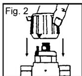
4. To limit the low temperature range at a set minimum (higher than pos. 1 to pos. 4): Place arrow on hand wheel as closely as possible to the right of the L-slot bracket (facing arrow). (fig. 2)
