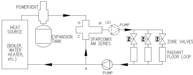
**CAUTION: DO NOT INSTALL PUMP BETWEEN CONNECTION "A" AND HEAT SOURCE.**
