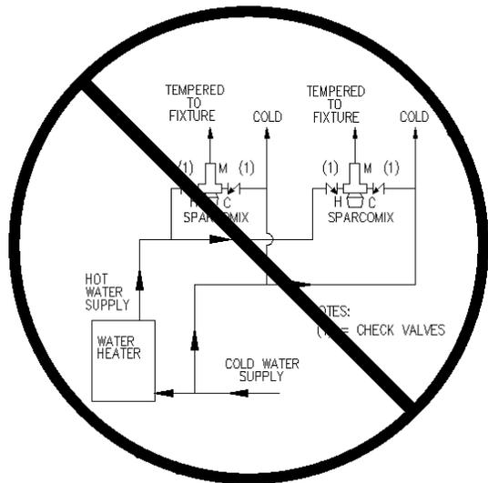
**DO NOT USE WHERE FURTHER BLENDING WITH COLD WATER WILL OCCUR. THIS TYPE OF INSTALLATION IS PROHIBITED.**
