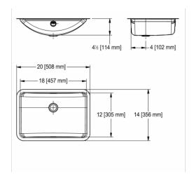
Single compartment undermount vanity basin. 18 gauge (1.2 mm), type 304 (CNS 18/10) stainless steel. Exposed surfaces are #4 satin finished. Undercoated to reduce condensation and resonance. Includes cutout template. Certified to ASME A112.19.3-2008 / CSA B45.4-08. Center back waste location, accepts 1 1/4" (32 mm) waste assembly (not included), integral overflow at front of bowl.
