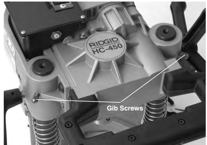
Figure 13 – Adjusting Gib Screws
