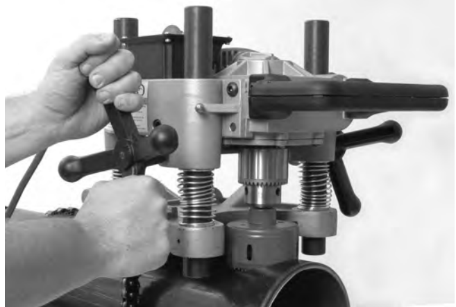
Figure 11 – Operating the Hole Cutting Tool
