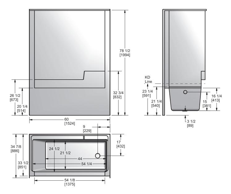
Measurement tolerances ± 1/4" (6.3 mm)
